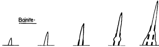
Figure 8: Schematic illustration of the edgewise growth mechanism of bainitic ferrite [27].
