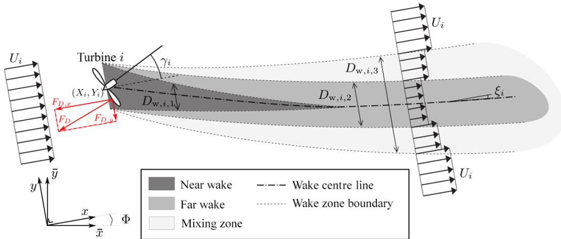
**Figure 1.** A schematic visualization of the wake model in FLORIS, containing three discrete wake zones. Furthermore, active wake deflection by purposely misaligning the turbine rotor with the flow is shown (cf. Fig. 4a in Gebraad et al., 2016).
