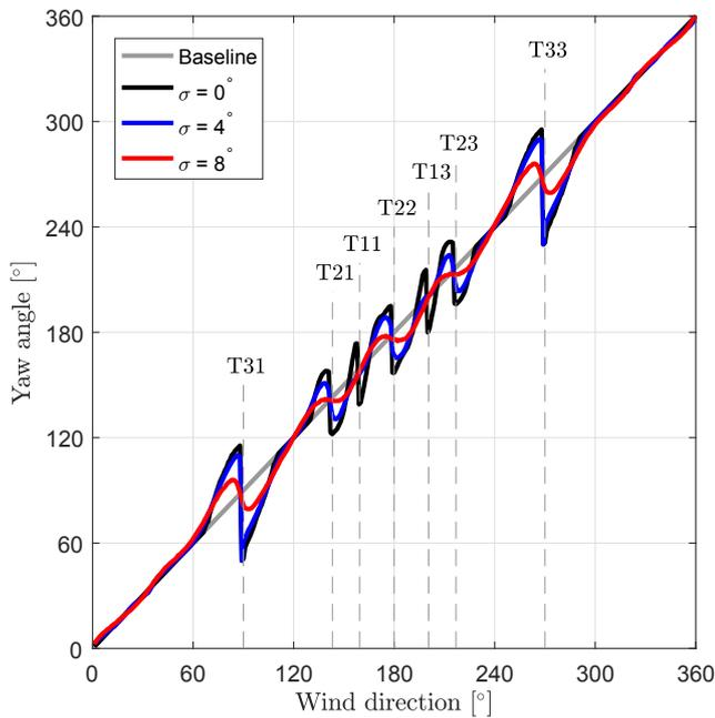
**Figure 6.** Optimized yaw angles of the centre turbine in the southernmost row (T32) for three different robustness parameters  $\sigma = 0$ , 4, and  $8^\circ$ . In addition, directions are marked and named accordingly, at which neighbouring turbines are located downstream.
