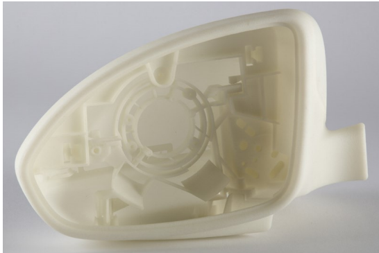
(a) Support for car side mirror printed with Polyamide via Selective Laser Sintering (Prodways, 2022)
