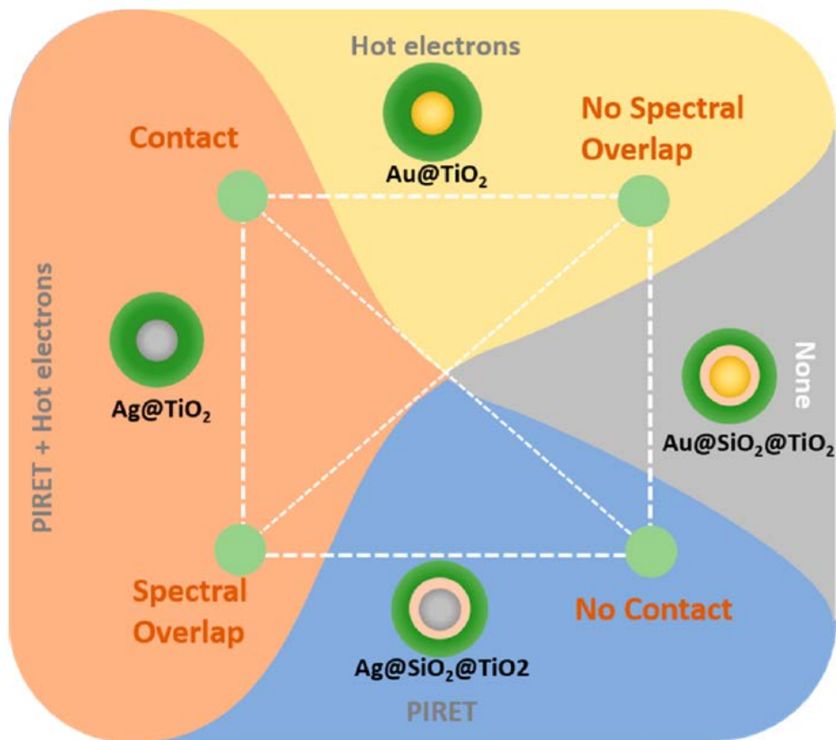
Figure 32. Variables that control the possible plasmonic enhancement near-field mechanisms for extending photoconversion. Connecting the line between the properties of the given core@shell nanoparticle gives the corresponding enhancement mechanisms present. Reprinted with permission from ref.[75] Copyright 2015 ACS.
