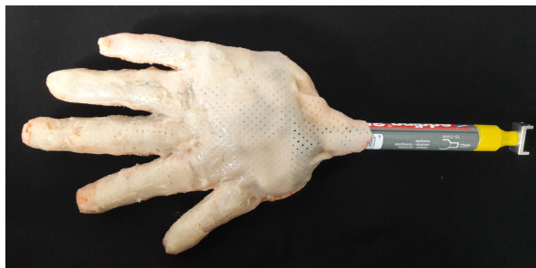
Figure E.1: Fabricated hand model to test the validity of the force calculations
