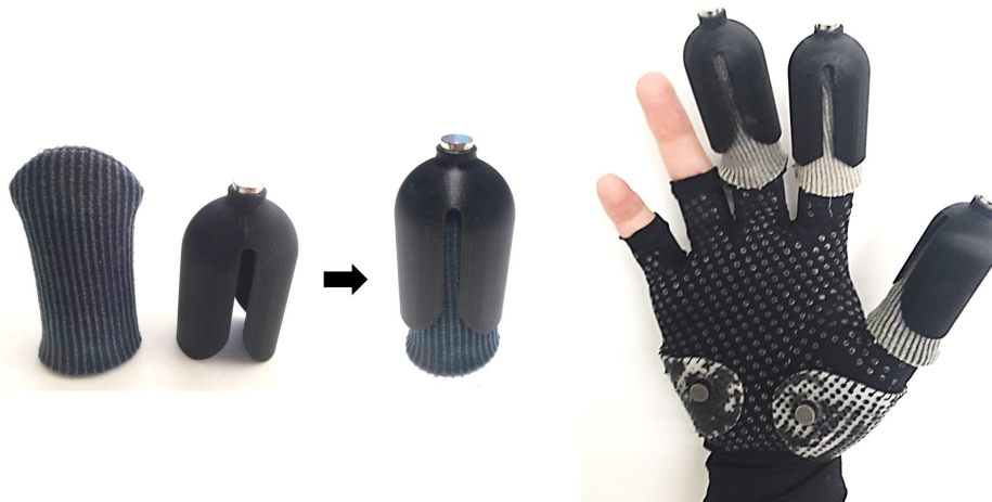
Figure A.2: Fingersleeves with magnetic tip to be worn on thumb, index and middle finger together with a fingerless glove with two additional magnets on the palm area.
