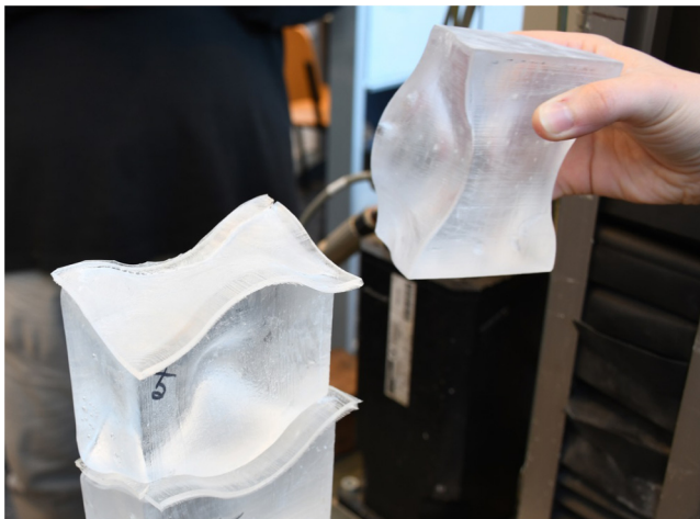
Fig. 33. Prototype of a 3 mm thick, cast interlayer from PU70 [30].
