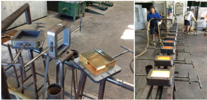
Fig. 6. High precision open steel moulds used for the manufacturing of the glass blocks for the Crystal Houses project.
