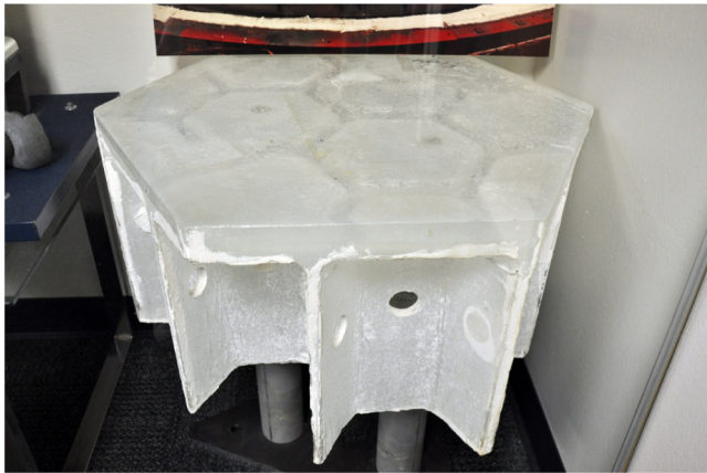
Fig. 15. Segment of the Giant Magellan's blank at the Steward Observatory, Arizona.
