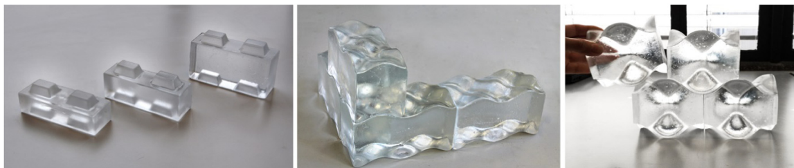
Fig. 35. Evolution of interlocking cast glass blocks towards more curved geometries of equal mass distribution. From left to right: interlocking glass brick inspired by the LEGO® block by [40], osteomorphic block by [42] and osteomorphic block by [30].
