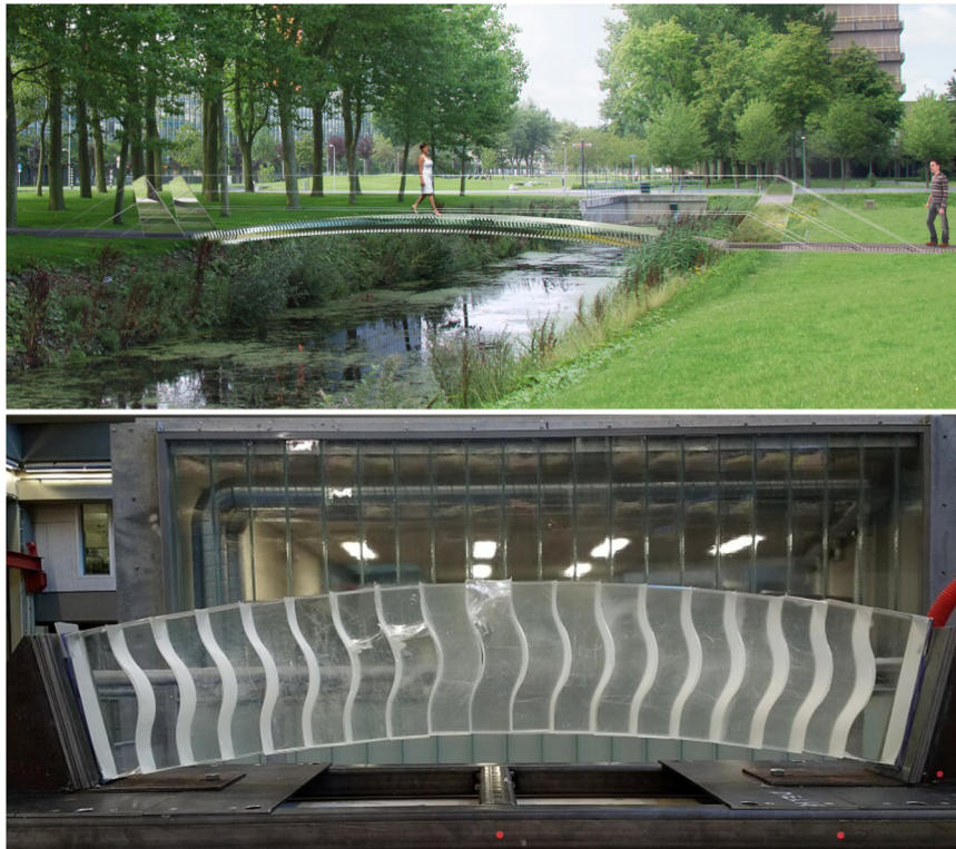
Fig. 34. Visualization (top) and a tested glass block prototype (bottom) of the dry-stacked glass arch bridge developed by [36].
