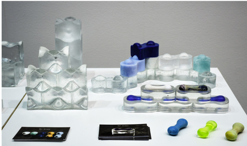
Fig. 36. Physical prototypes of different interlocking geometries by [30].
