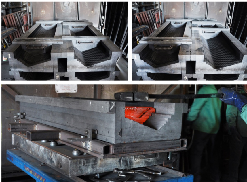
Fig. 7. Adjustable graphite mould at John Lewis Glass Studio for the components of the Ice Falls project by James Carpenter.
