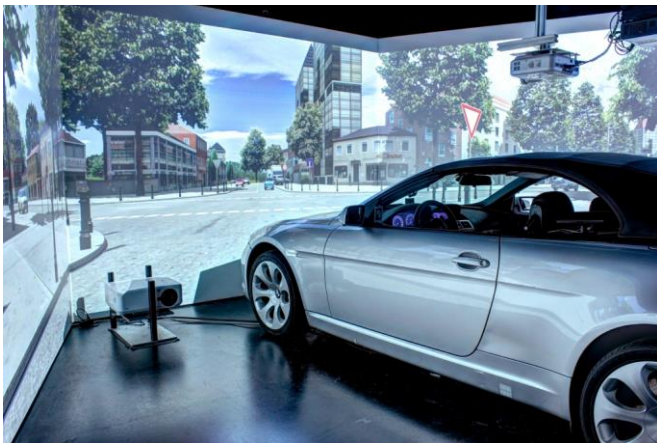
Figure 1. The high fidelity driving simulator used for the experiment.
