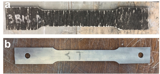
Fig. 2. Tensile specimens cut from WAAM plates: (a) as-printed and (b) after surface milling.
