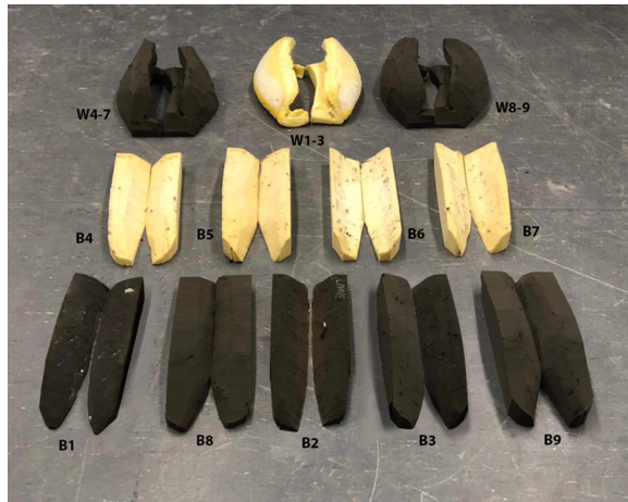
Figure 3.2: An overview of the bolster and wing designs in the study.
