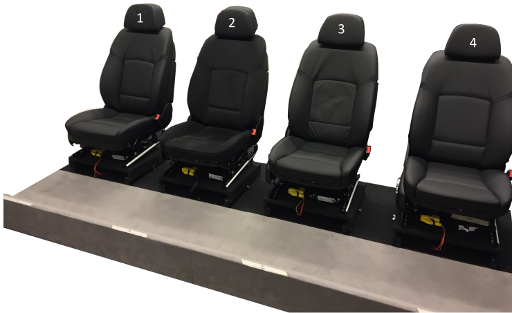
Figure 7.1: The figure illustrates the setup of the study with all four seats in a row from left to right: reference seat (seat 1); Alcantara seat (seat 2); loose cover tension (seat 3), and the seat with the metal plate instead of the seat suspension (seat 4).
