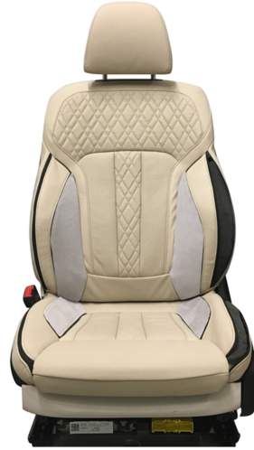
Figure 3.1: Modified BMW 5-series set with zippers and exchangeable foam inserts and cover material.
