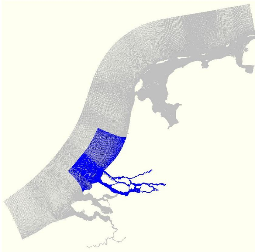
**Fig. 4.1.:** Flow grid Voorne (blue) nested in the *kuststrook* flowgrid (grey).
