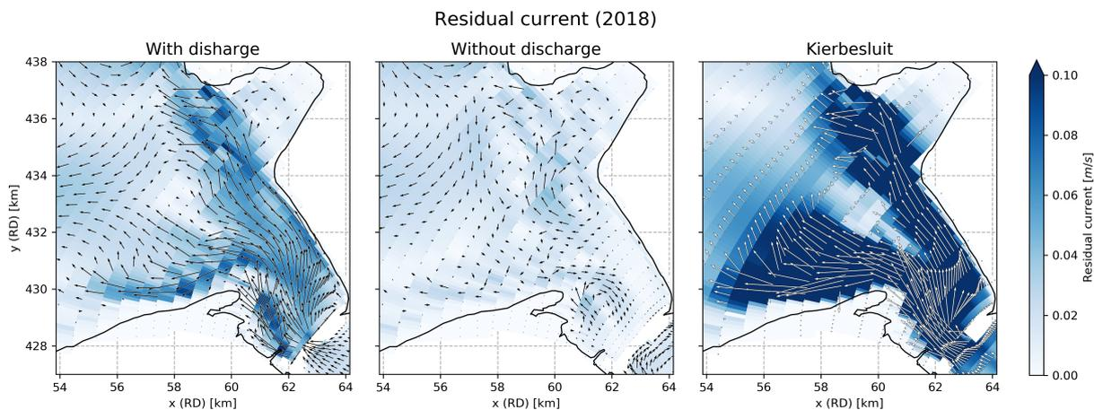
**Fig. 6.8.:** Residual current during different sluice policies (2018).
