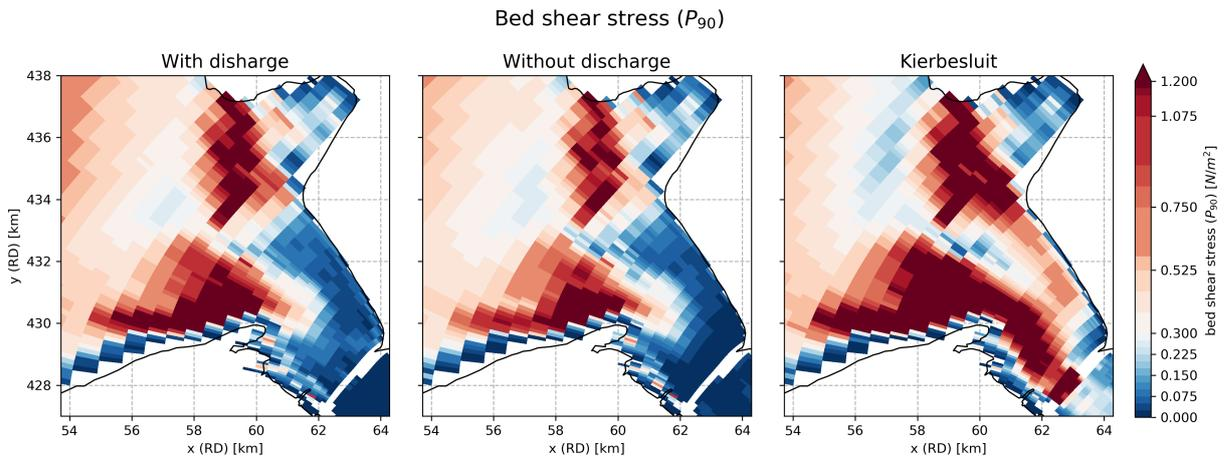
Fig. 6.10.: 90<sup>th</sup> percentile bed shear stress during different sluice policies (2018).
