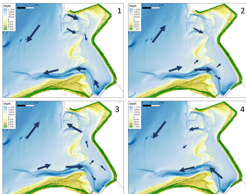
**Fig. 2.6.:** Propagation of the tide in the study area after construction of the Haringvliet sluice (Drawn after Cleveringa (2006c)).
