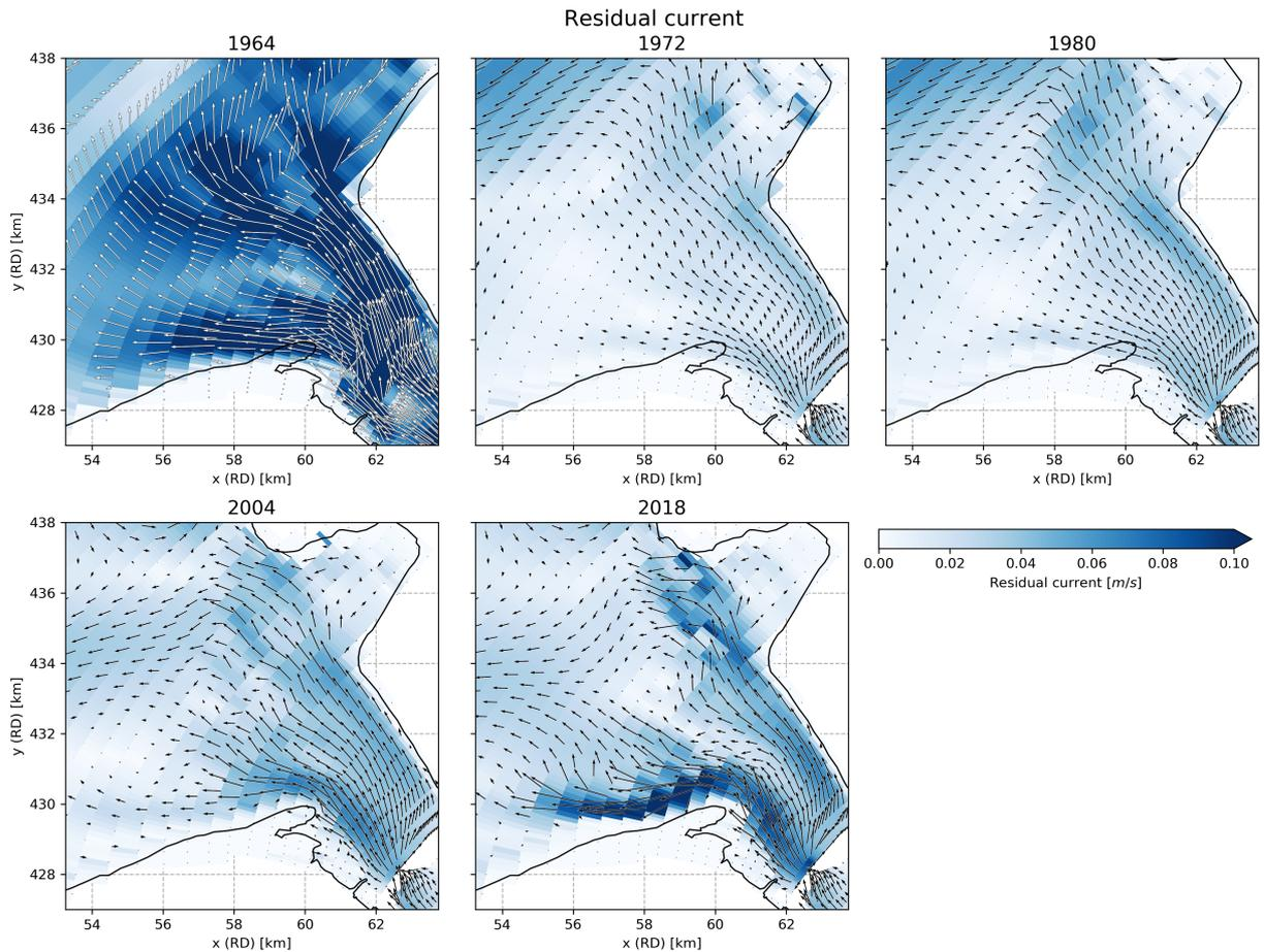
**Fig. 6.7.:** Residual current per stage in time.
