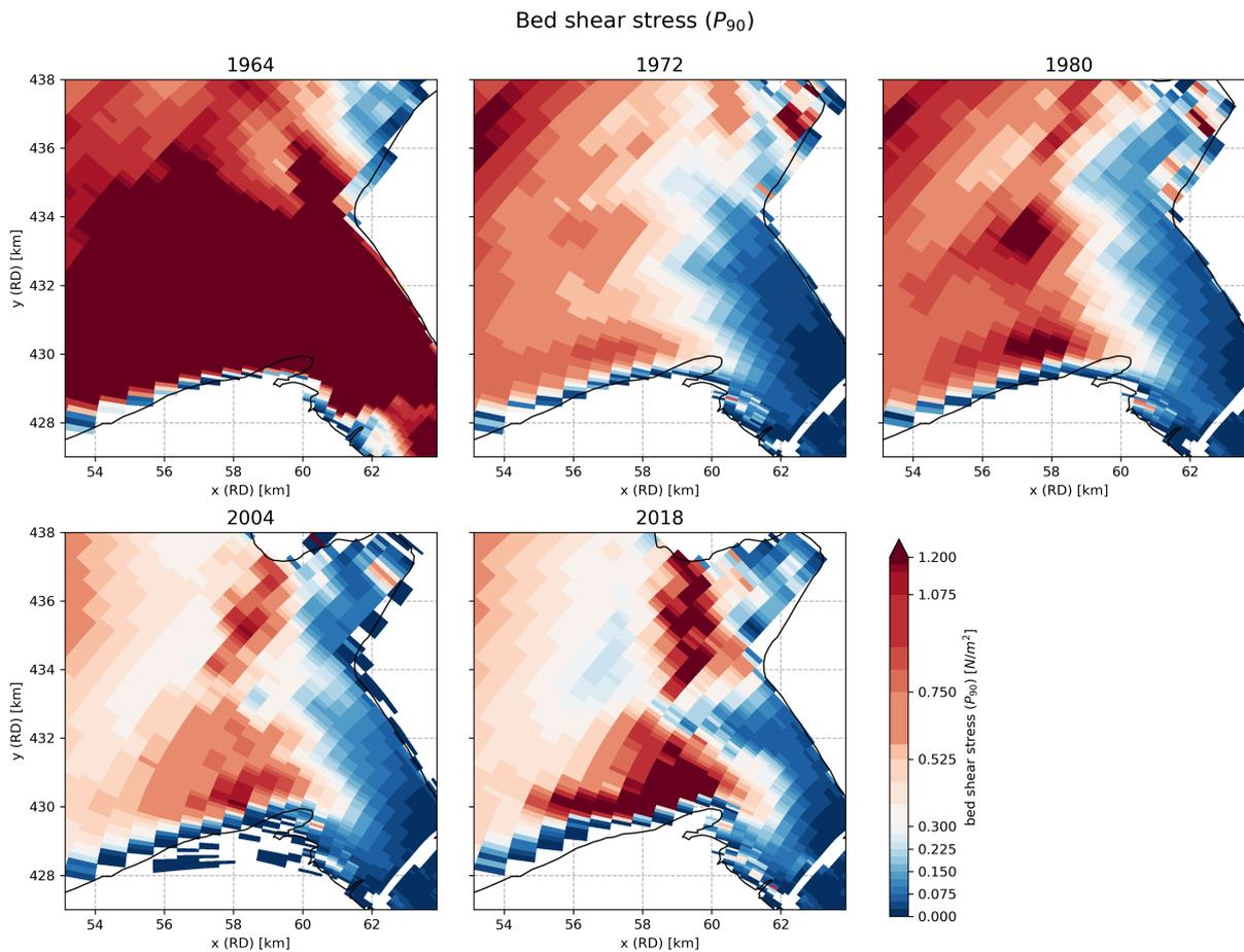
**Fig. 6.9.:** Bed shear stress per stage in time.
