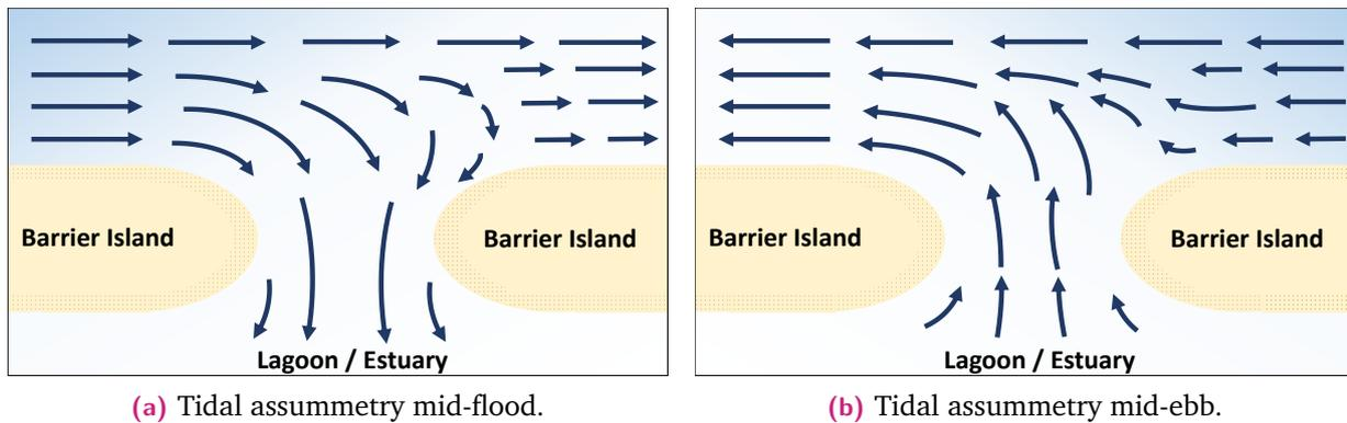
**Fig. 2.3.:** Tidal asymmetry ebb tidal delta (Redrawn after Sha and Van den Berg (1993)).
