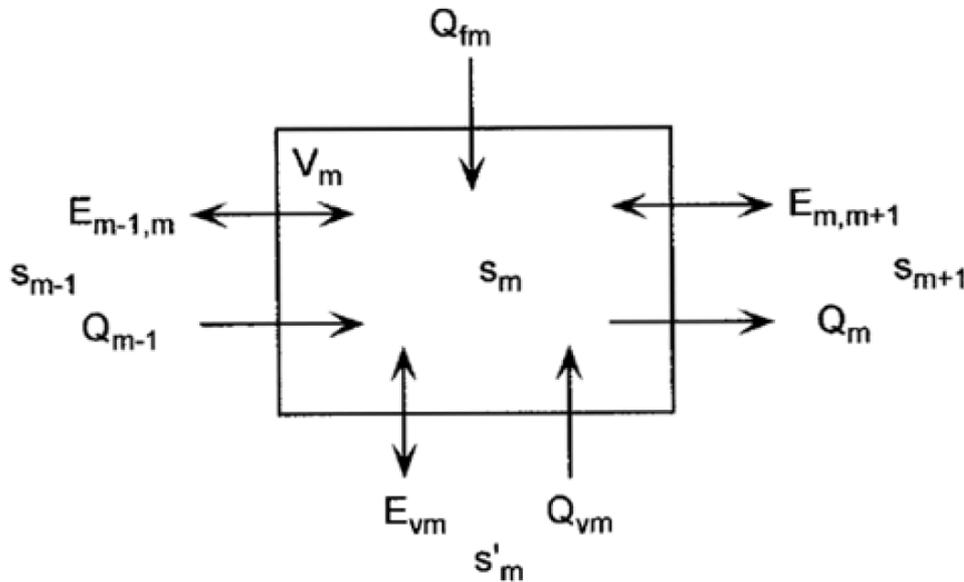
**Fig. A.3.:** Schematization of salt water exchange for a two layer estuarine box model (Hagy et al., 2000).
