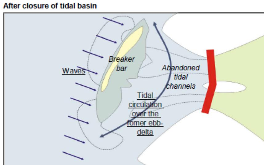
Fig. 2.5.: Schematisation of the Haringvliet after closure (Cleveringa, 2008).
