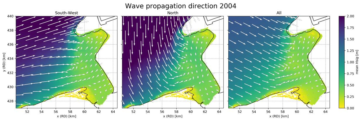
**(d)** Wave propagation direction 2004.
