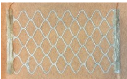
Figure 4. Disposable on-skin sensor with wave pattern
