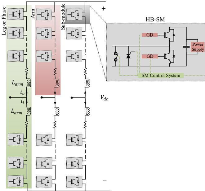
Fig. 1. MMC configuration with HB SM.
