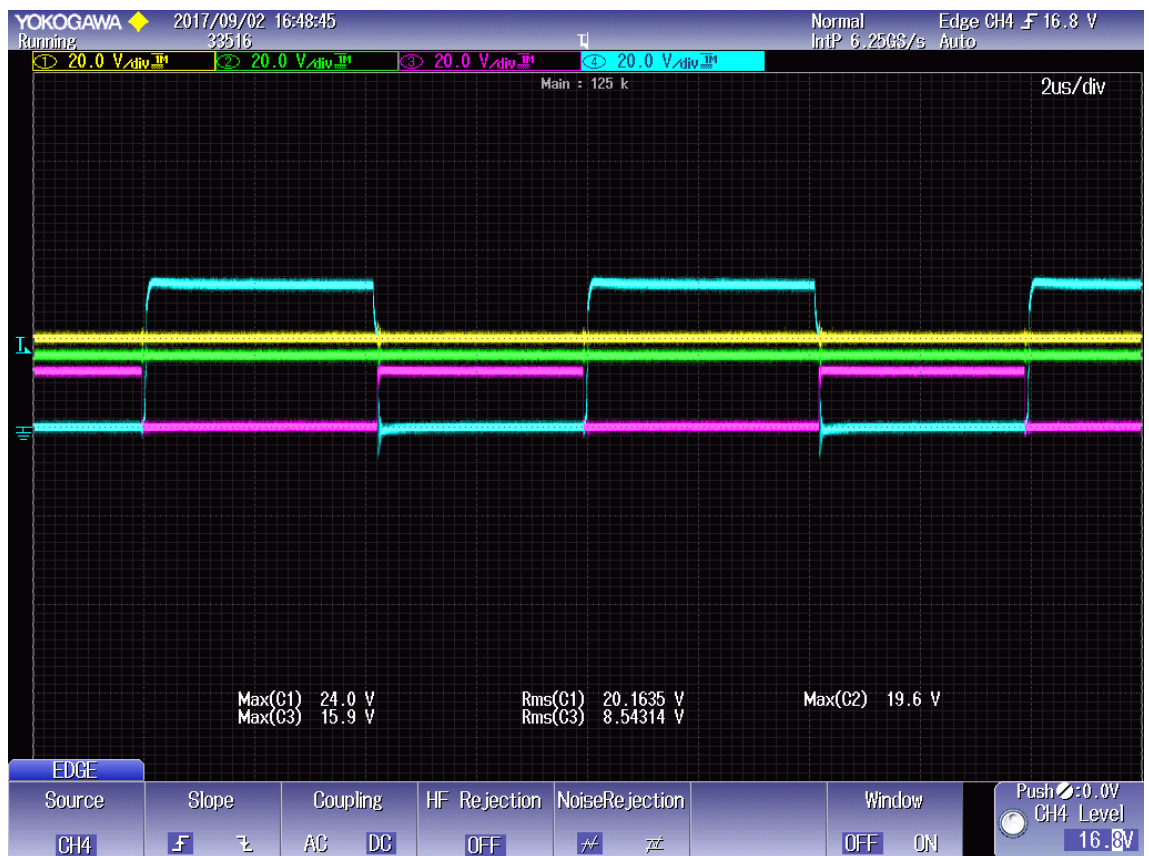
Figure 80. 9.06VDC link- 20V output switching scheme
