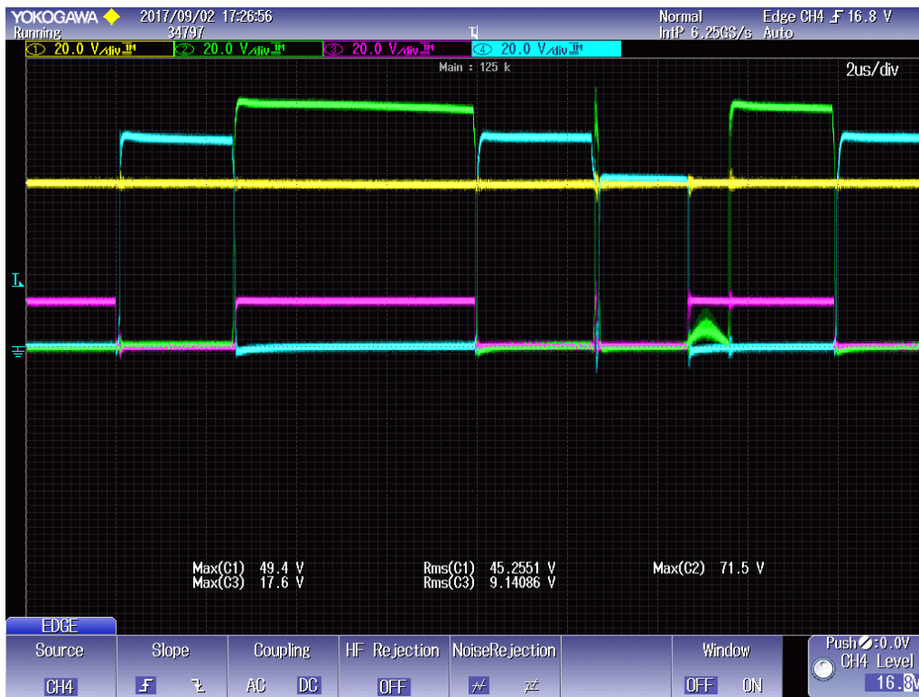
Figure 85. 48VDC link- 48V output switching scheme
