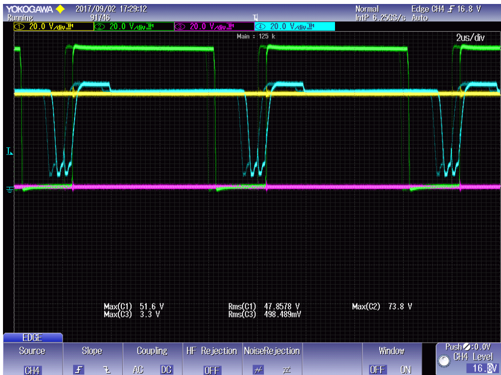
Figure 86. 60VDC link- 48V output switching scheme
