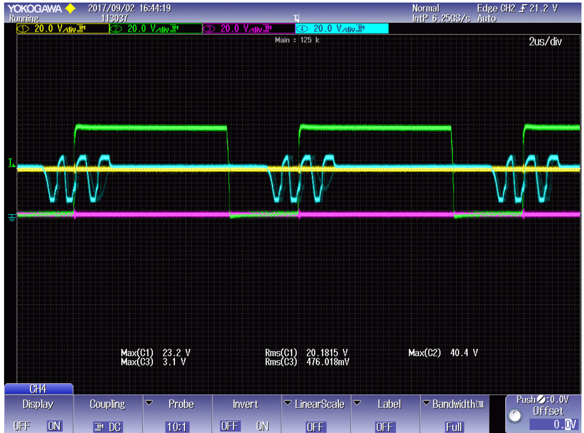
Figure 83. 30VDC link- 20V output switching scheme
