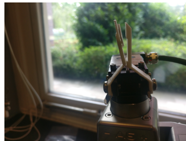
Figure 6.9: Grippers not closing
