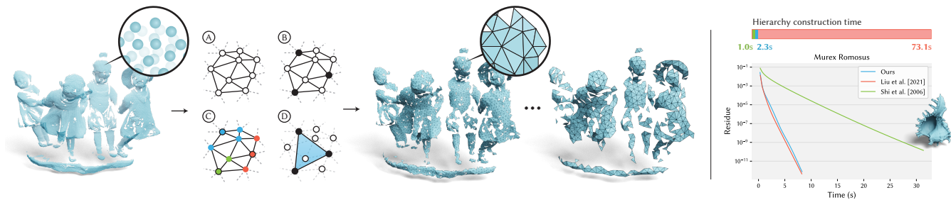
Figure 1: Illustration of our hierarchy construction for one level. Starting from a mesh or point cloud, A) we construct a neighbor graph on the surface. B) We then sample a spatially uniform set of nodes, C) compute the graph Voronoi diagram of the samples, and D) project unsampled points onto triangles formed by edges between Voronoi neighbors. This is repeated for every level. Right: Comparison of run time for solving a Laplace system on a triangle mesh. Our hierarchy construction is fast, while achieving similar solver performance to the state-of-the-art.
