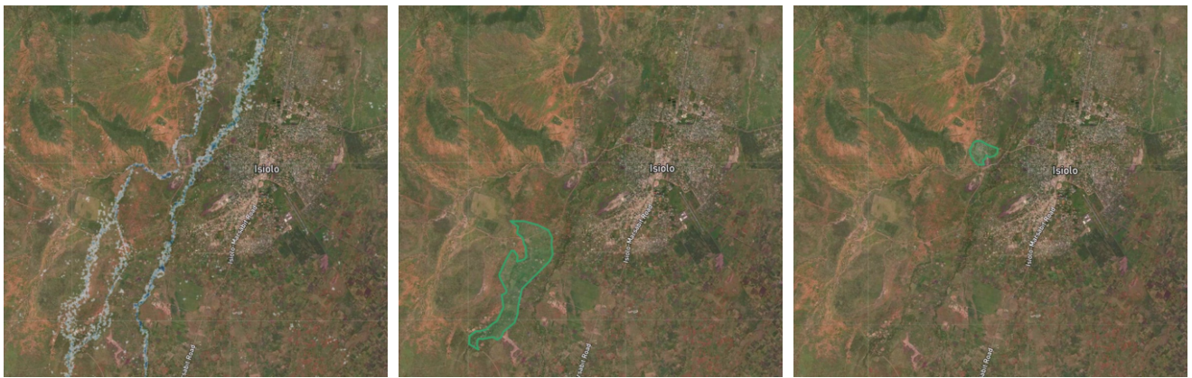
(a) Flood map displayed in FIS Tool Interface (b) Agricultural land protected from 1 meter water depth (c) Residential area protected from 1 meter water depth
