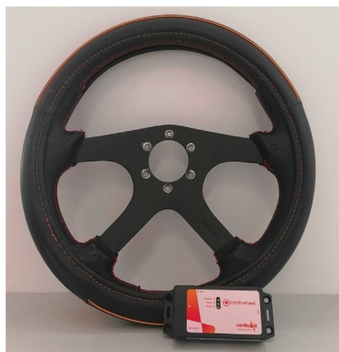
Fig. 1. CardioWheel for collecting drivers' electrocardiogram and lead on detection signals.
