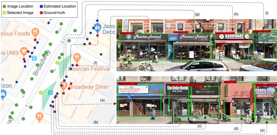
Figure 2.4: Qualitative results of our integrated approach on detecting, classifying, and mapping storefronts using street-level imagery
