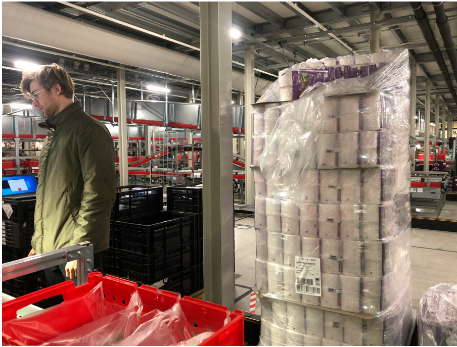
Figure F.8: Some items, like toilet paper, needs to be unpacked from a pallet before picking. This adds picking time and energy.
