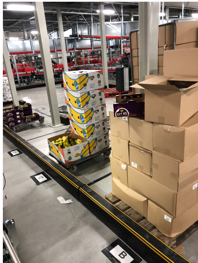
Figure F.5: Another example of manual item reslotting. Shoppers place one box of mangoes closer to the station, resulting in virtually no walking time for every 10 mangoes that are picked. This figure also shows large height differences between item pick locations. This is not taken into account in the task decomposition.
