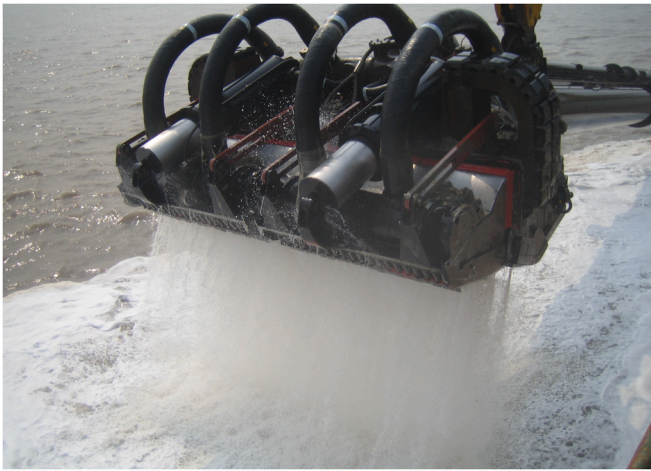
Fig. 1. Draghead with nozzles of a trailing suction hopper dredger (Image courtesy of Boskalis).
