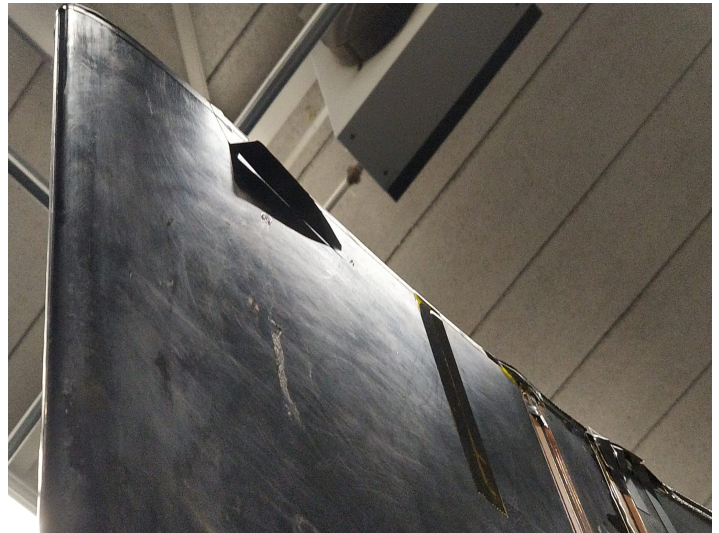
(b) Loose tape discovered on the bottom surface near the wing tip.
