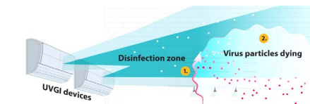
Figure 43 Visualization of upper-room UVGI for air purification (photocatalysis)
