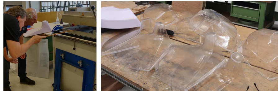
Figure 85 Vacuum forming top and bottom hood in 1/4 pieces at the PMB, TU Delft
