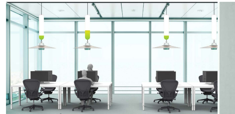
Figure 97 CADR distributed amongst multiple Personal Air Filter's to reduce the fan speed and thereby noise produced
