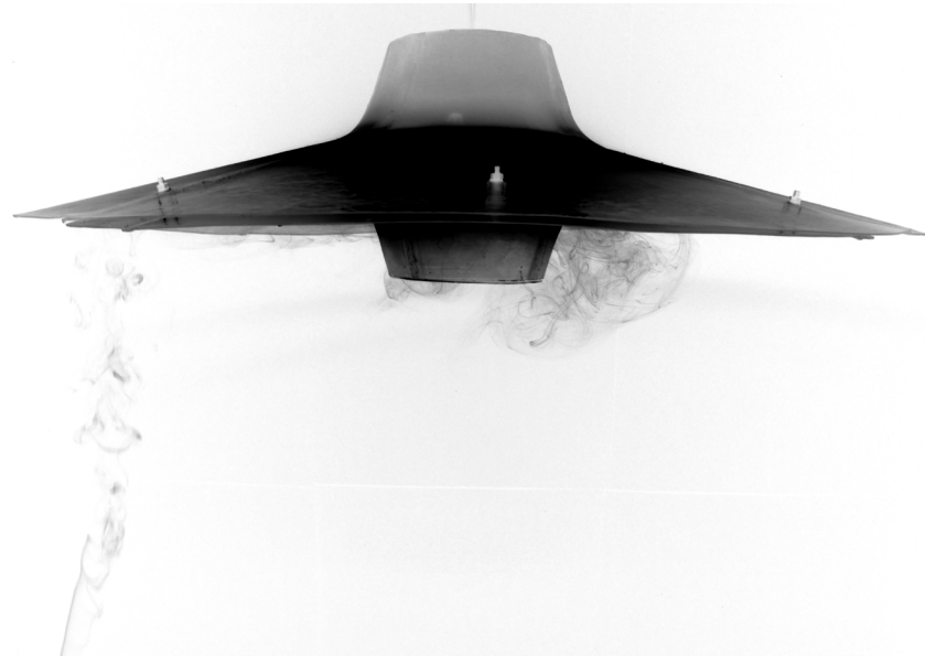
Figure 117 Smoke buildup underneath hood of the Personal Air Filter (50m 3 /h) (inverted colour)
