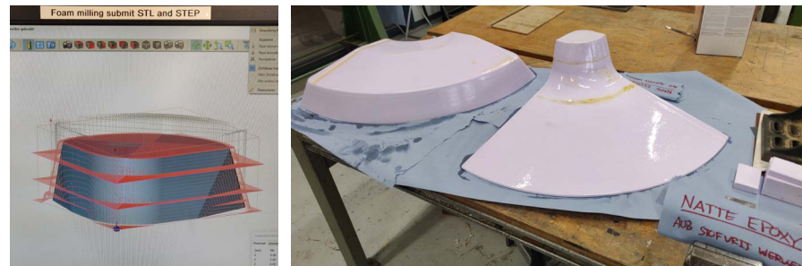
Figure 84 Milling foam moulds for hood, and preparing them with laminar epoxy coatings
