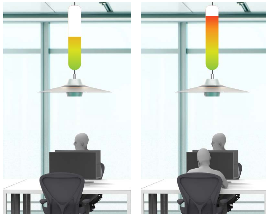
Figure 95 Smart-mode fan speed for one person (left) or multiple people (right)
