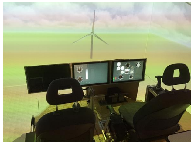
Figure 20 ONERA PycsHel simulator including the NREL5MW wind turbine.
