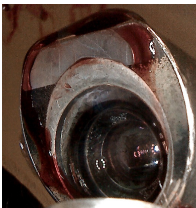
Fig. 8 Laparoscope lens tip contaminated due to blood (Aarts, 2015)
