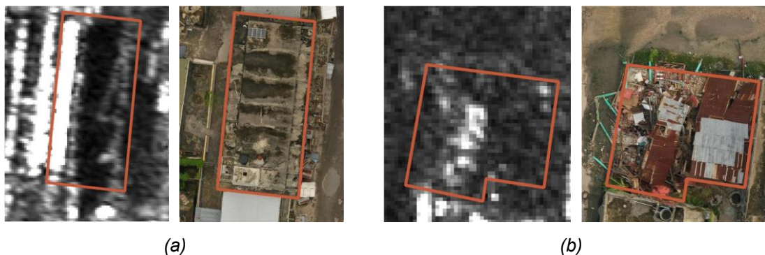
Figure 1: Examples of (a) an intact building in VHR SAR data and drone orthophoto and (b) a collapsed building in VHR SAR data and drone orthophoto. The VHR SAR data is Capella imagery acquired over Les Cayes, Haiti (  2021 Capella Space All Rights Reserved).
