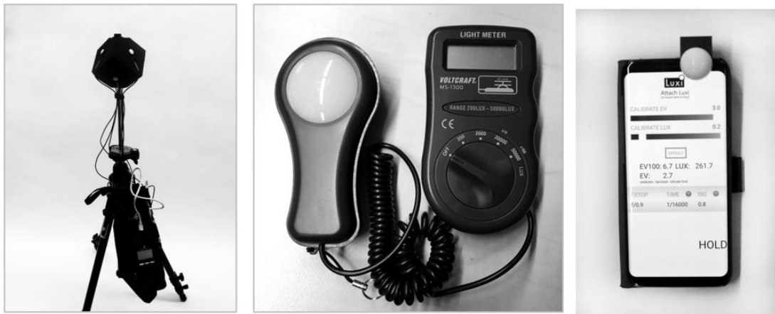
Figure 13 Measurement devices. Left to right: cubic meter based on the Konica Minolta system, 32,53 luxmeter and smartphone with Luxi
