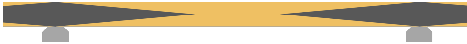
Figure 1.4: Impression of the gradual transition of timber (brown) to steel (dark grey).
