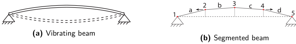
Figure 4.1: Vibration of a hinged-hinged beam
