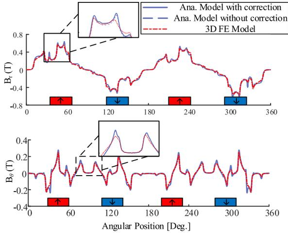
Fig. 16. Total MFD waveforms under angular misalignment.
