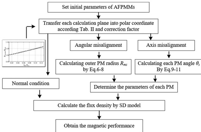
Fig. 28. Calculation flowchart.
