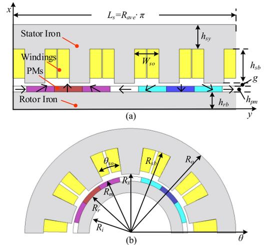
Fig. 3. Analytical model for AFPM machine. (a) Analytical model in Cartesian coordinates. (b) Converted model in polar coordinates.
