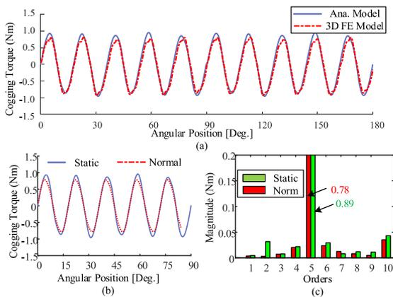
Fig. 17. Cogging torque under static angular misalignment condition. (a) Waveforms. (b) Comparison. (c) Harmonics.
