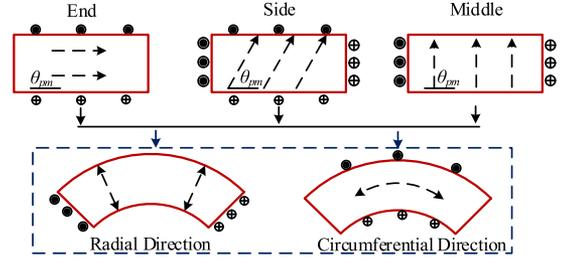
**Fig. 6.** PM under different magnetization.
