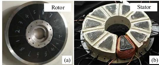
Fig. 2. Configuration of the AFPM machine. (a) Rotor. (b) Stator.
