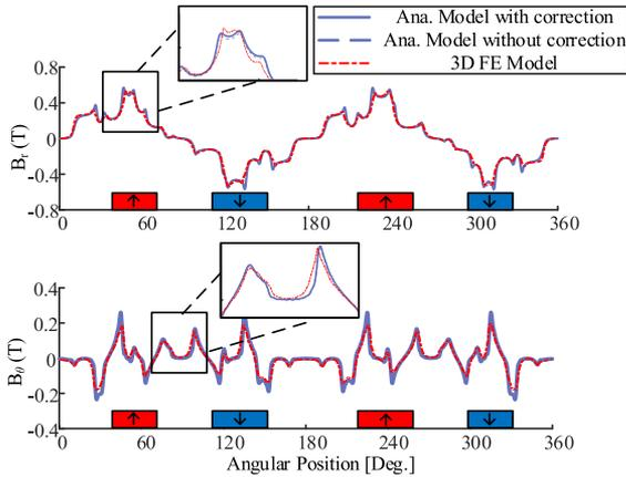
Fig. 21. Total MFD waveforms under angular misalignment.
