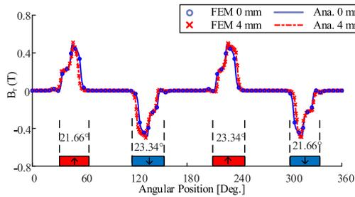
Fig. 20. Total MFD waveforms under axis misalignment.
