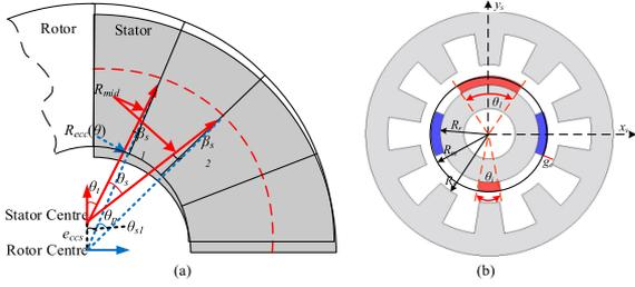
Fig. 9. (a) Configuration of axis misalignment. (b) Axis misalignment illustration under polar coordinate.
