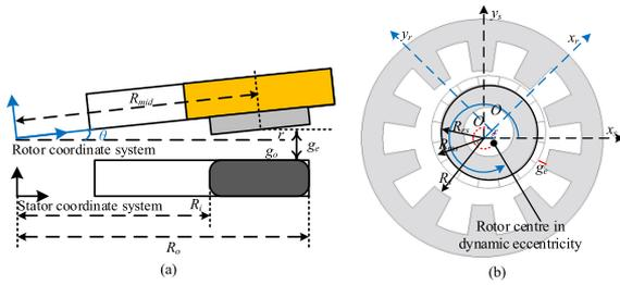
Fig. 7. (a) Configuration of angular misalignment. (b) Angular misalignment illustration under polar coordinate.
