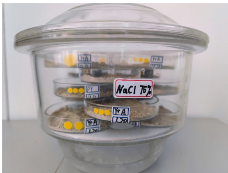
Fig. 2. The setup for cement pre-hydration.
