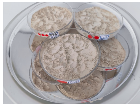
Fig. 2. The setup for cement pre-hydration.
