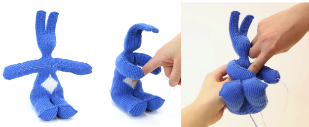
Figure 8: The Bunny by Albaugh, Hudson and Yao [3] is an example of morphic textile-forms that changes in use-time. The knitted form has both tendons and sensors integrated within the machine-knitting process which could enable the arms to hug. Image credit: Lea Albaugh, Scott Hudson and Lining Yao
