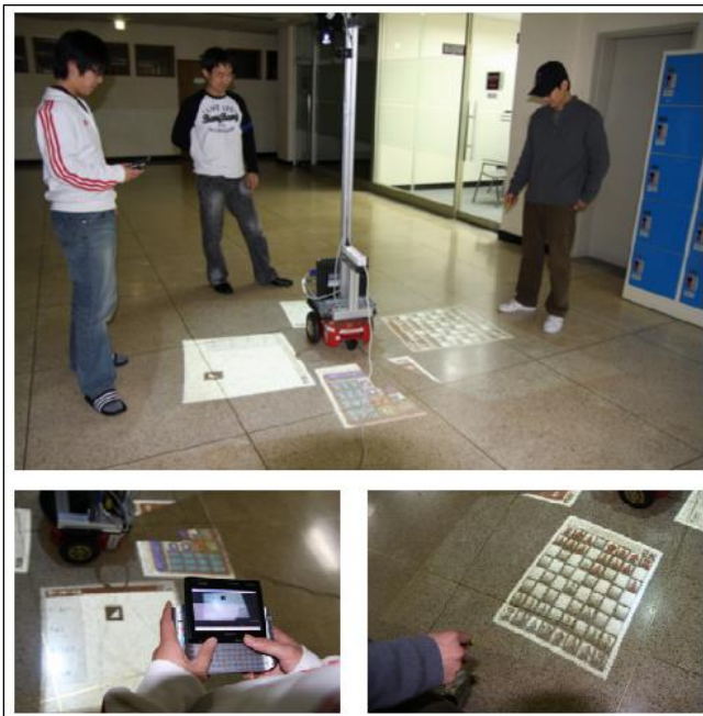
Image 35: an experimental setup by Covert [69] shows the user which obstacles have been perceived by the AGV. The system makes distinctions between short term, mid term and long-term problems and assigns visual cues which signal an appropriate amount of urgency.
