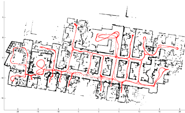
Image 12: Thousands of SLAM measurements together form a map. For AGVs a 2D map is sufficient but a 3d map is also possible. The map contains both static points (such as walls and permanent obstructions) as well as temporary points such as humans or other AGVs. Image adapted from [19].
