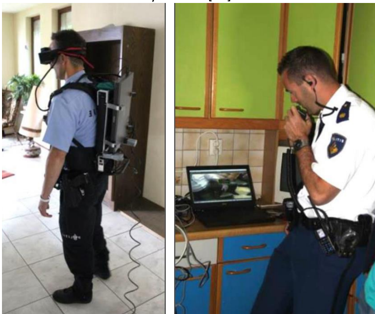
Image 29: Image adapted from Lukosch & Lukosch [60]. Two policemen are virtually co-located using an AR HMD. The remote colleague can highlight suspicious objects in the scene or point in the direction of emergency exits.
