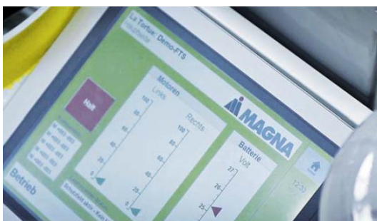
Image 25: The screen on prototype 1 shows additional information such as the values of the sensors and the status of the AGV.
