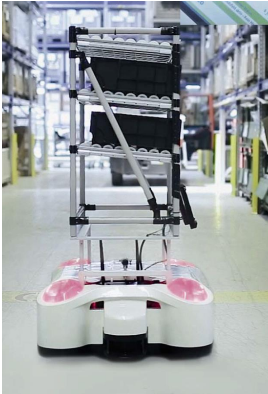
Image 24: Magna AGV Prototype 1 in action with a storage delivery rack mounted as a modular attachment.
