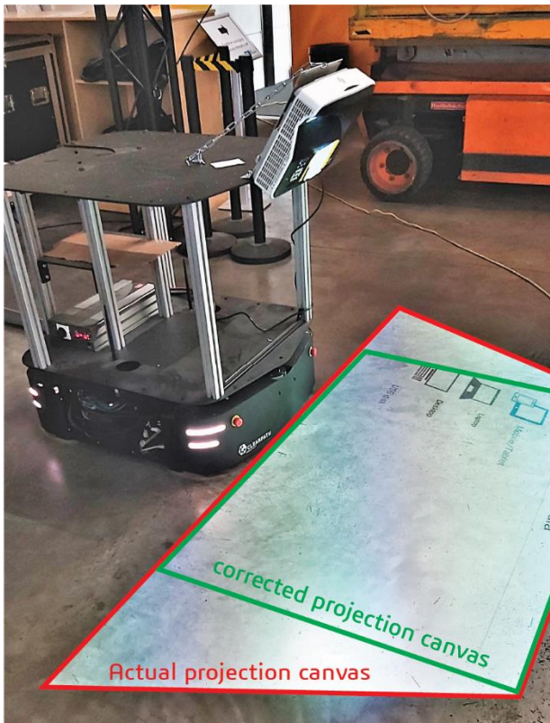
Image 41: Because the projector is not mounted perfectly perpendicular to the floor the projection is warped. The red line indicates the actual projection canvas. The green line indicates the corrected canvas.
