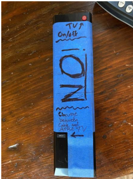
Image 19: The physical equivalent of a "diminished reality". The TV remote has all buttons that are not needed covered with tape to minimize confusion and misuse. Image source: Reddit.
