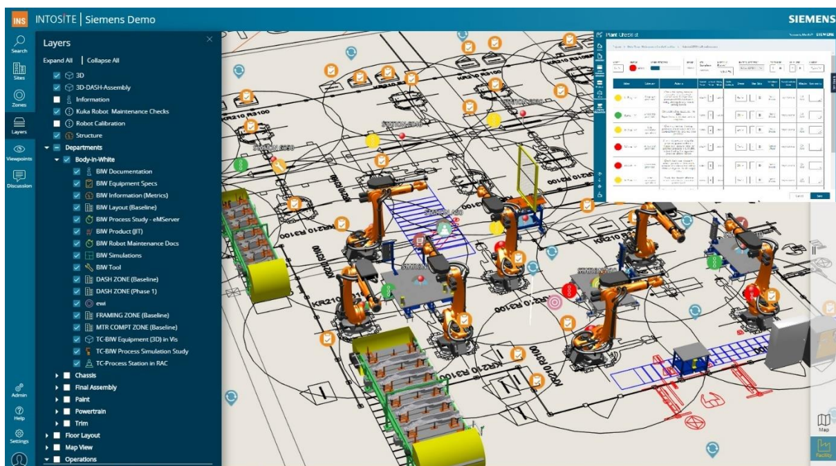
Image 5: an example of a digital factory by Siemens [8]. AGV locations, assembly lines states, and the positioning of every robot arm are included.
