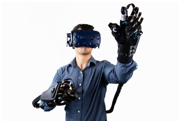
Image 18: In virtual reality, senses are blocked off in order to be replaced. In this picture we see a man use an HTC Vive for visual VR, a headset for auditory VR and HapTX haptic gloves for haptic VR.
