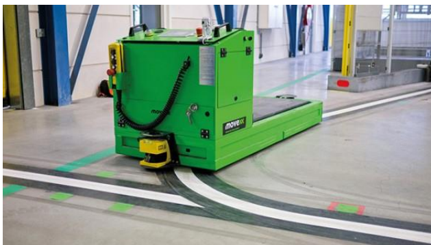
Image 9: An AGV system that uses painted navigation lines. Source: Movexx.com.
