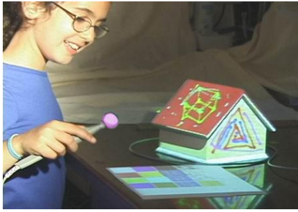
Image 20: This 2001 project called Shaderlamps [45], [46] explored a variety of tabletop applications to apply colors and textures to real-life objects using projectors.
