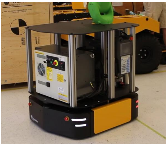
Image 62: Most AGV's (like this ridgeback AGV) that are used in a factory context have indicator lights just like cars. They are used to communicate intent or the robot's current status.
