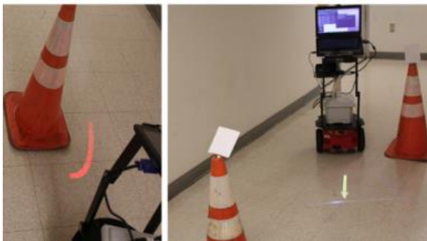
Image 35: an experimental setup by Covert [69] shows the user which obstacles have been perceived by the AGV. The system makes distinctions between short term, mid term and long-term problems and assigns visual cues which signal an appropriate amount of urgency.
