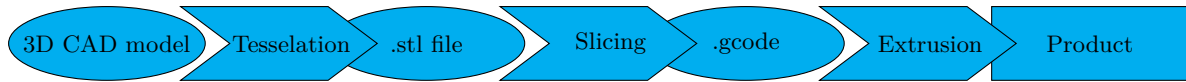
Figure 1.17: Flow diagram from CAD to final product in the Fused Deposition Modeling process
