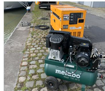
Figure 4.9: Air Compressor &amp; Power Unit
