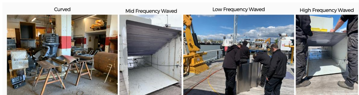
Figure 4.12: Different ramp designs during experiments
