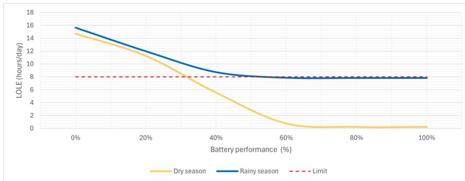
Figure 9.5: Loss of Load Expectation hours with battery performance during a day
