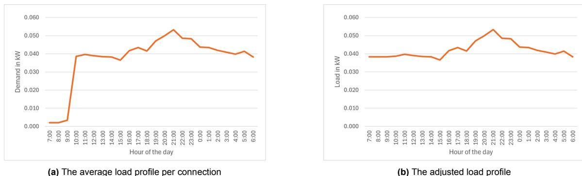
**Figure D.3:** The original and adjusted load profile per connection
