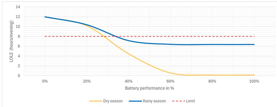
Figure 9.6: Loss of Load Expectation hours with battery performance during the night
