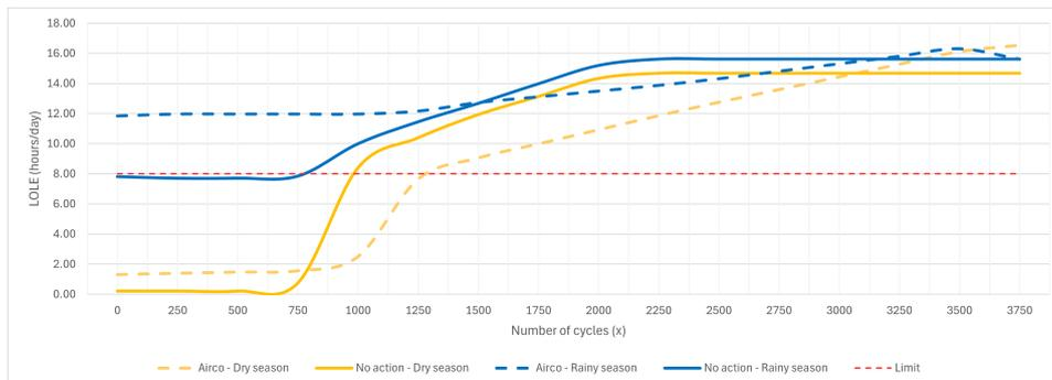
Figure 9.15: Lifetime battery with and without air conditioning
