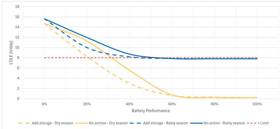
Figure 9.16: Loss of Load Expectation additional battery capacity for a day
