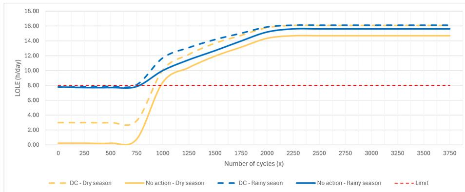
Figure 9.12: Lifetime of battery with and without DC
