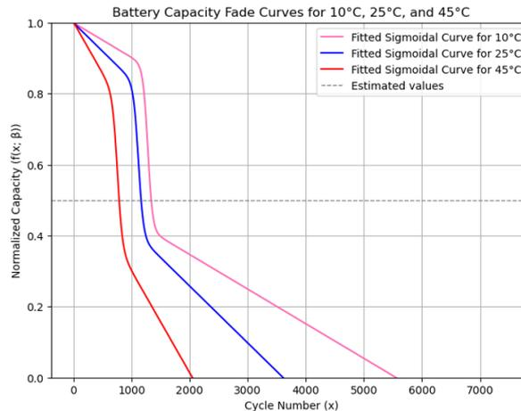
**Figure 6.2:** The capacity fade curve under different temperatures used [68]
