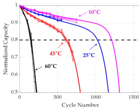
Figure D.5: Capacity fade curve battery under different temperatures [68]
