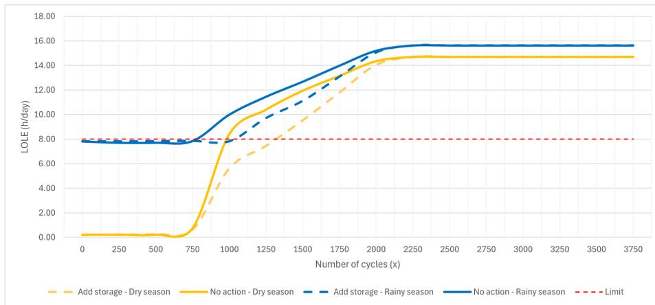
**Figure 9.18:** Lifetime battery with and without additional battery capacity in both seasons
