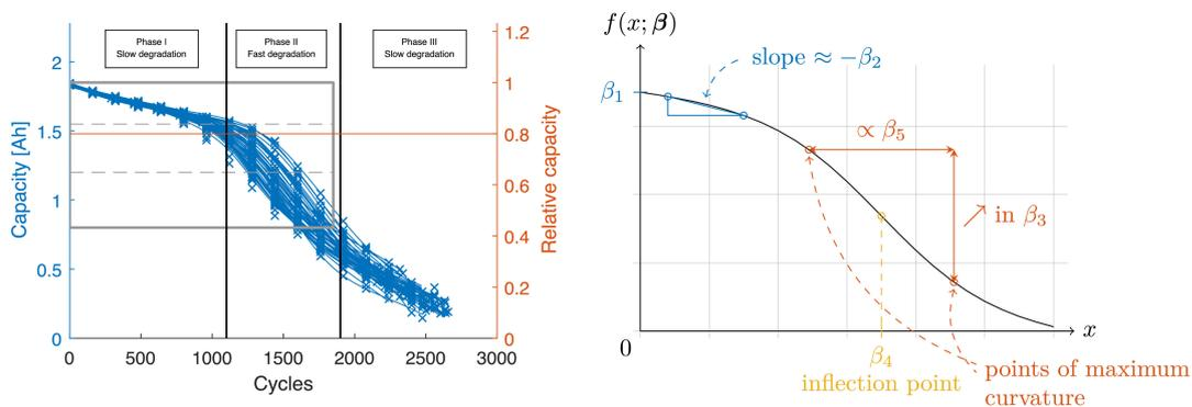
Figure D.4: Capacity fade curve battery including parameters [70]
