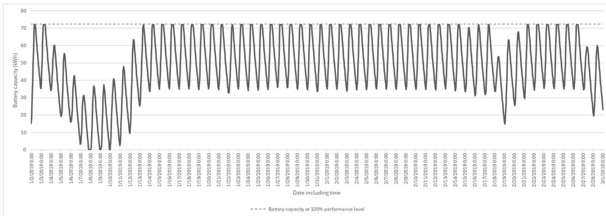
Figure 9.3: State of Charge battery in dry season for January and February
