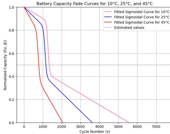
**Figure D.6:** Extrapolation of capacity fade curve battery under different temperatures
