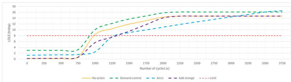
Figure 9.24: Overview of battery lifetime in the dry season for the experiments
