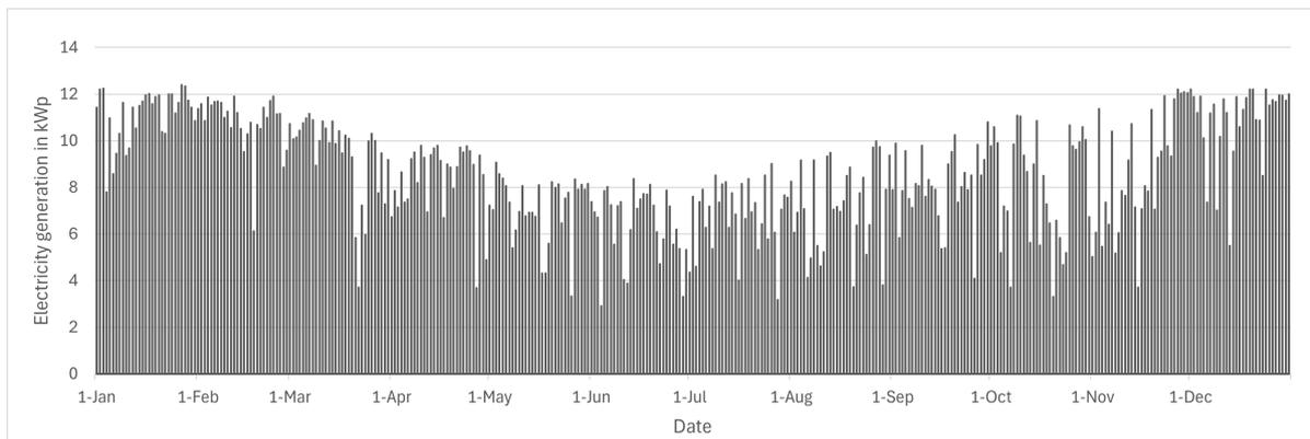
**Figure 8.2:** Generation profile of a 16 kWp micro-grid
