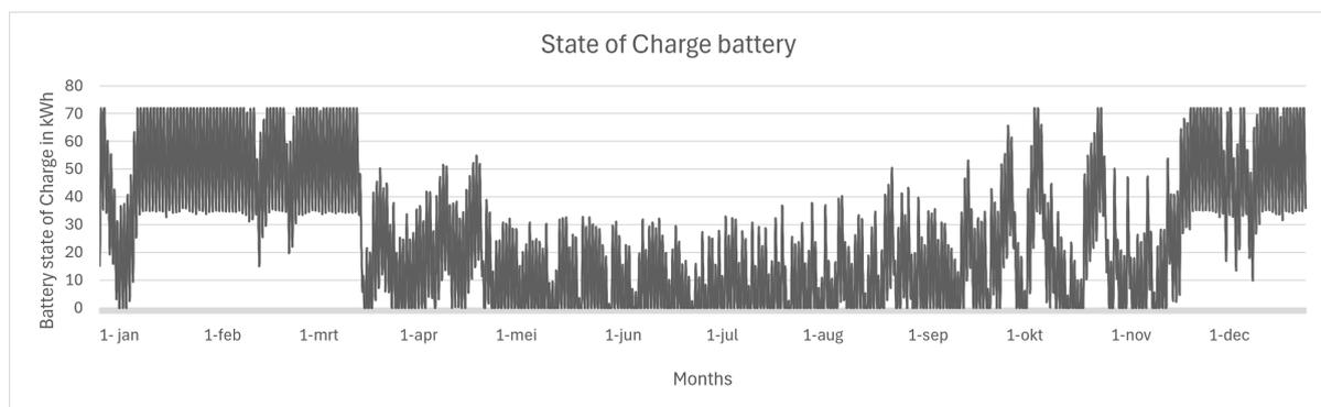
**Figure 8.4:** State of Charge of the micro-grid battery
