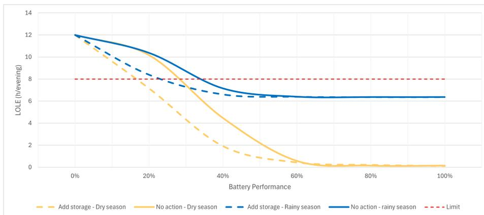
Figure 9.17: Loss of Load Expectation additional battery capacity for a night
