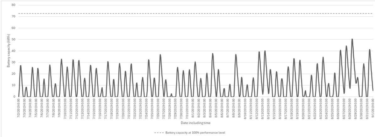
Figure 9.4: State of Charge battery in rainy season for July and August
