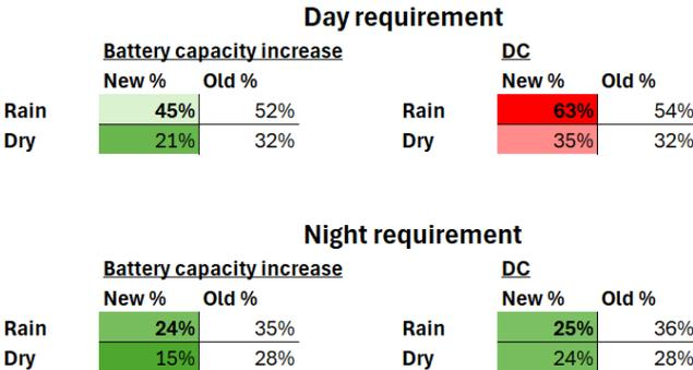
Figure 9.25: Minimal battery performance percentage to meet system requirements
