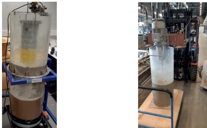
Figure 1. Left: A picture of the laboratory setup. A transparent cylindrical tank was filled with the following layers: sand at the bottom, a bentonite suspension, and water. Right: A picture of the drill used to homogenize the bentonite suspension.
