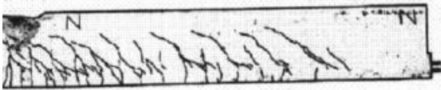
Figure 5-31; Right part of the crack pattern of experiment VS-C3
