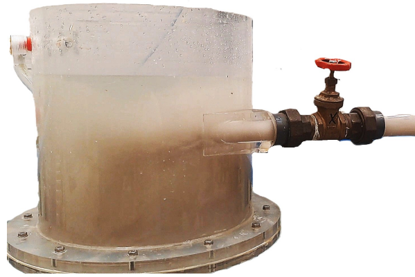
Figure 5.9: Coarse sediment (B-series): Solid separation in the hopper
