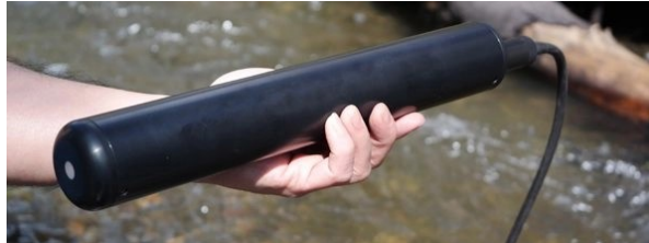
Figure 3.4: Acoustic backscatter sensor [42].
