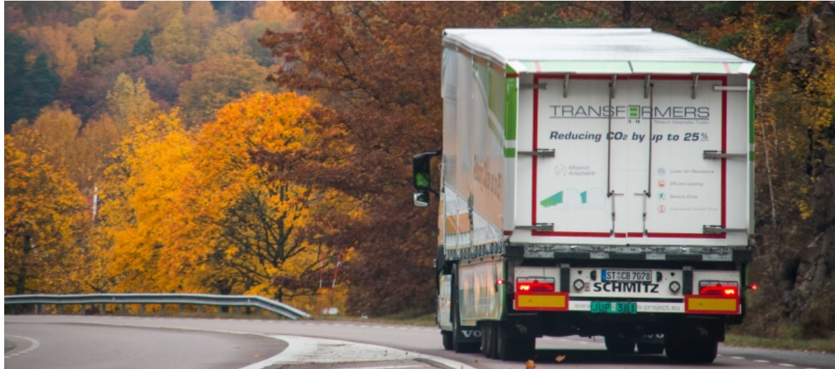
Figure 7.1: Road test of a variable trailer geometry concept reducing the height at the rear of the trailer combined with a boat tail. Source: TRANSFORMERS [62]
