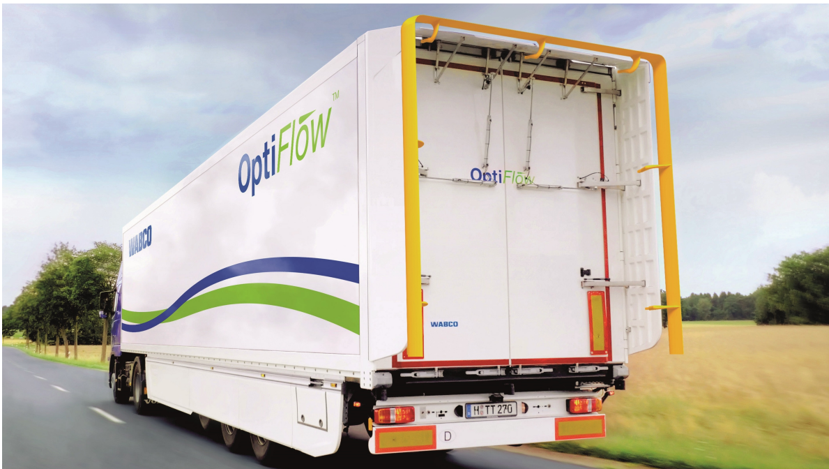
Figure 1.8: Concept of combining a HDV tail and a guide vane. Source: Edited from Wabco [69]
