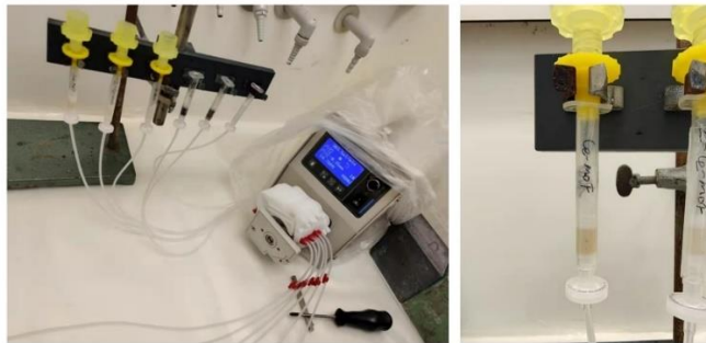
Figure S4.2. Photos of column experimental set up (left) and the fabricated column (right).
