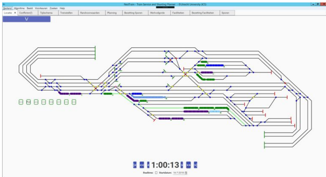
Figure 3.12: The Graphical User Interface of HIP. The black lines are the track of the node and the trains are represented in different colors (a color represents a rolling stock type). The time is represented underneath and can be changed by the buttons left and right of the time.
