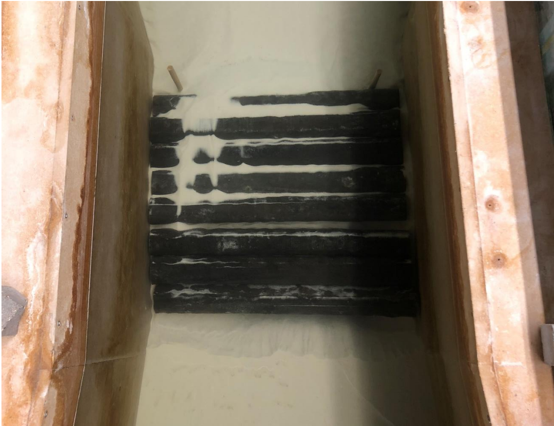
Figure 90; Uniform scour hole causes logs to roll in
