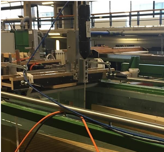
Figure 11; Vectrino (black cylinder marked 2), attached to a pulley device, mounted on a movable cart
