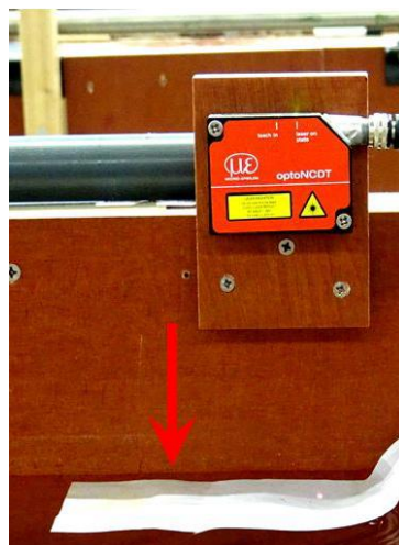
Figure 9; short range laser in combination with reflective floating paper (Stenfert 2017)
