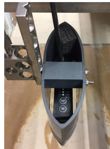
Figure 10; long range laser mounted inside a boat, with a clear glass bottom
