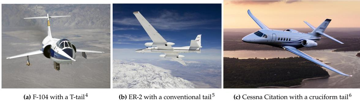
**Figure 5.2:** Three tail configurations compatible with wing-podded engines
