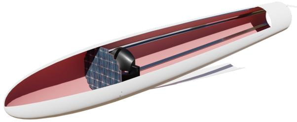
Figure 6.3: Weather radar in ESRA wingpod
