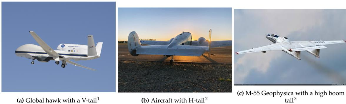
Figure 5.1: Three tail types potentially compatible with centrally mounted engines
