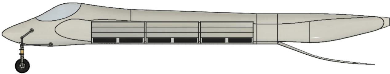
Figure 6.7: ESRA's offloading ramp for the payload pallets
