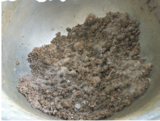
Figure 6G2: Growth of fungus in soil cow-dung mix prepared with dry cow-dung
