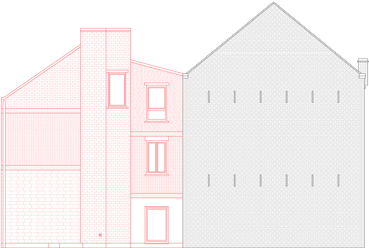
Figure 12, facade drawing of the side wall of house extension Mortsel with its collage of bricks and bonds (own work)
