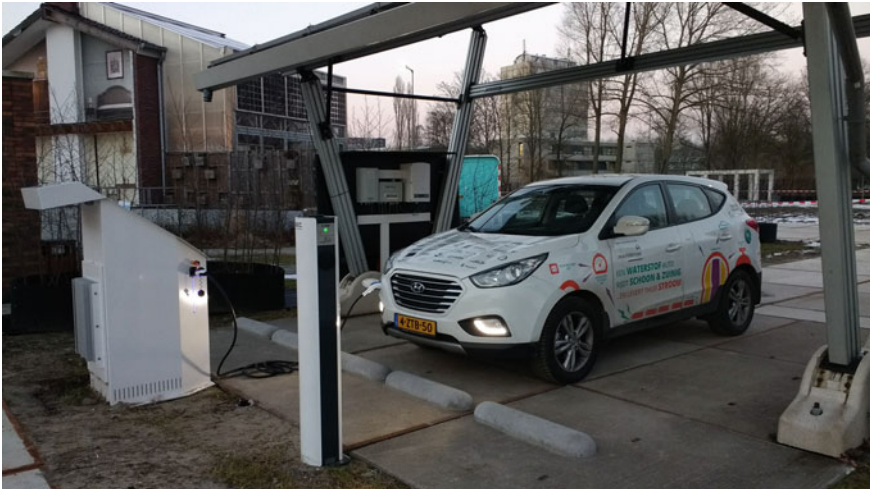
Fig. 8.3 Photo of the modified Hyundai ix35 FCEV connected to the grid through the V2G unit at The Green Village in The Netherlands
