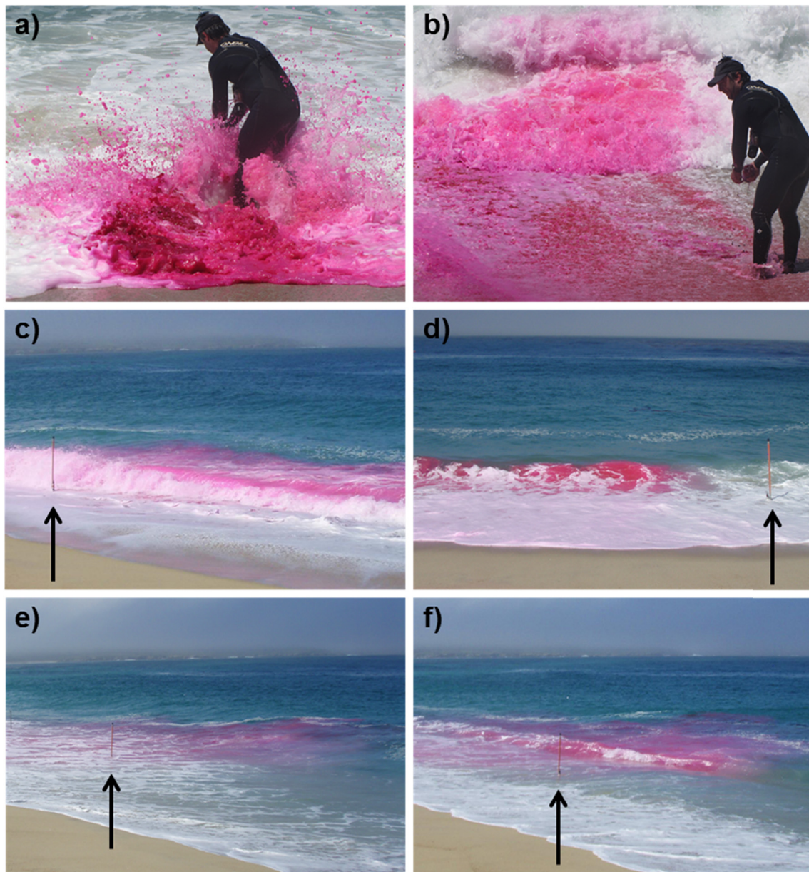
Fig. 3. Photos showing examples of (a) the initial dye slug release, (b) the well-mixed surf/swash zone shortly after the dye release, (c–d) turbulence and mixing of dye at the shoreline by breaking waves and alongshore advection of dye within the surfzone, and (e–f) run-down colliding with an incoming breaking wave resulting in the dye seeping offshore. Black arrows indicate locations of poles with dye sensors attached near the sea-bed in the surf zone, where (c–d) the intermittency of the dye observations is highlighted as the sensor is alternately submerged and not submerged.
