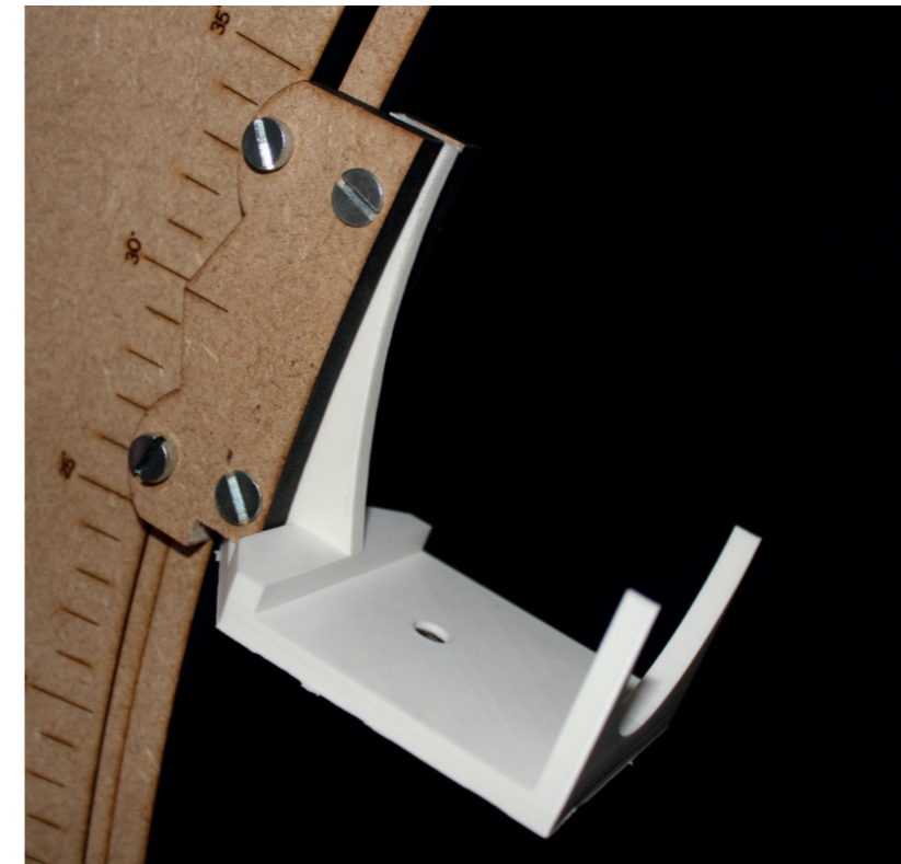
Fig. 5.9: The 3d-printed camera holder clamped on an arm
