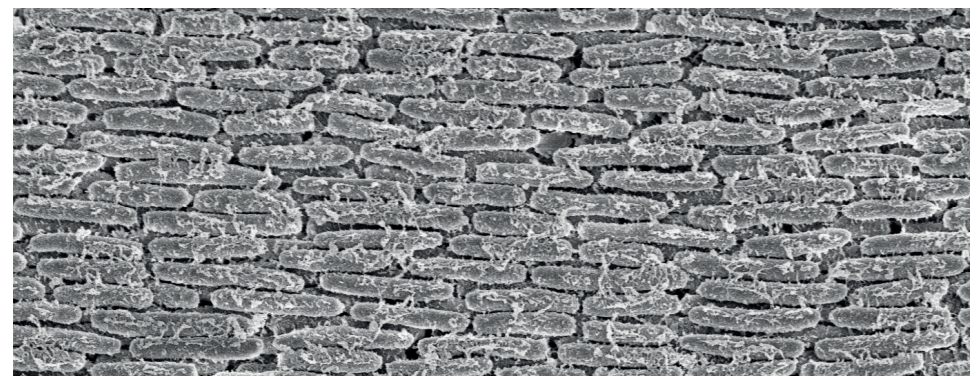
Fig. 2.12: Electron microscopy showing the highly ordered cells packed in a photonic crystal (Hoekmine B.V., 2020b)
