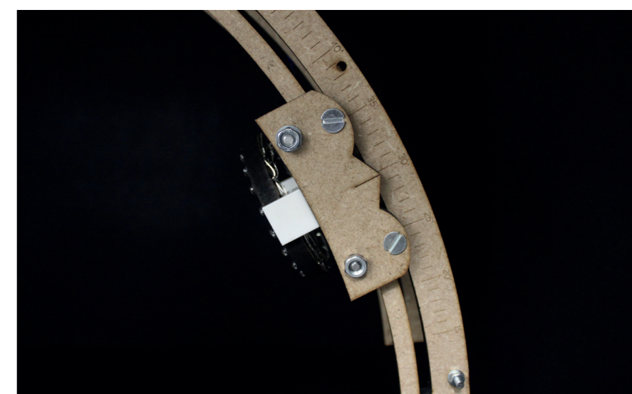
Fig. 5.3 [top]: The LED ring illuminating the petri dish Fig. 5.5 [middle]: The LED ring connected to the moving LED arm Fig. 5.6 [bottom]: The adjustable altitude angle of the LED ring
