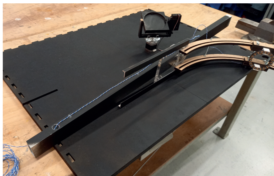
Fig. I.14: Electric wires of the LED ring connected to and going through the aluminium profile
