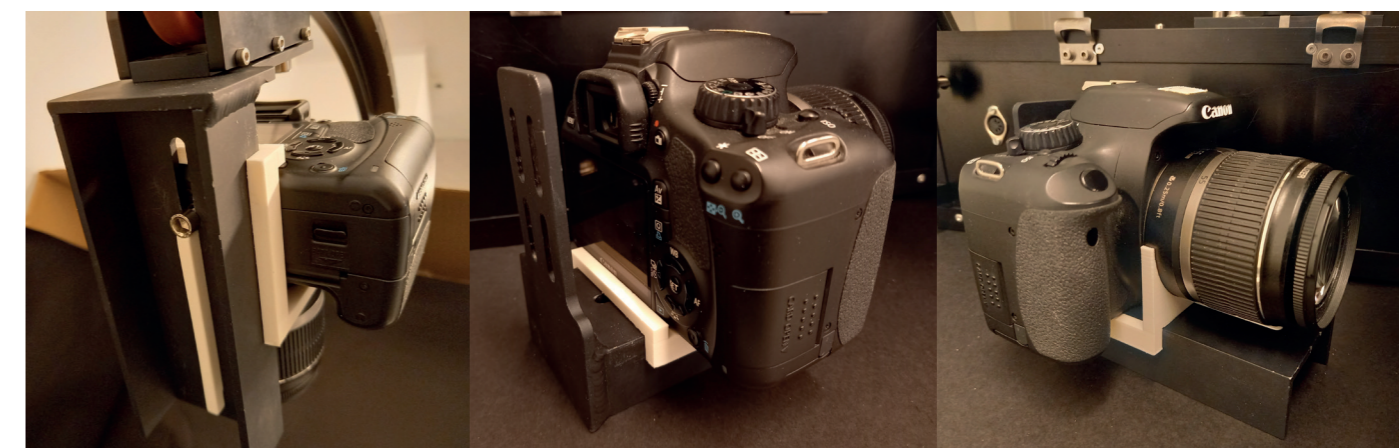
Fig. F.1 [bottom]: The 3D printed camera holder Fig. F.2 [right top]: The gonioreflectometer setup Fig. F.3 [right]: The LED mounted to the setup
