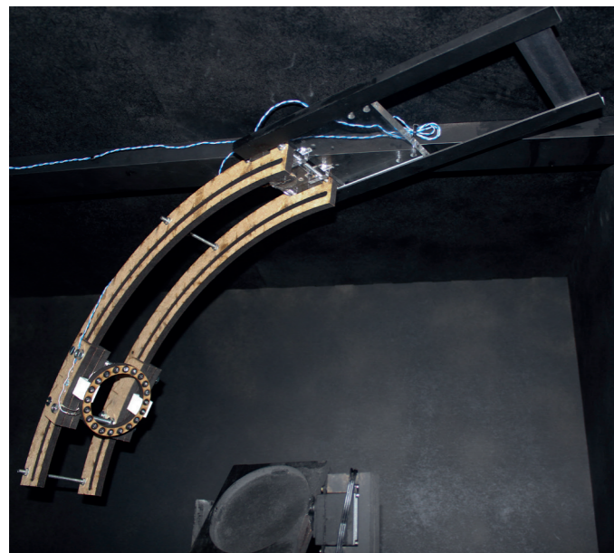
Fig. 5.7: The counterweight connected to the moving LED arm
