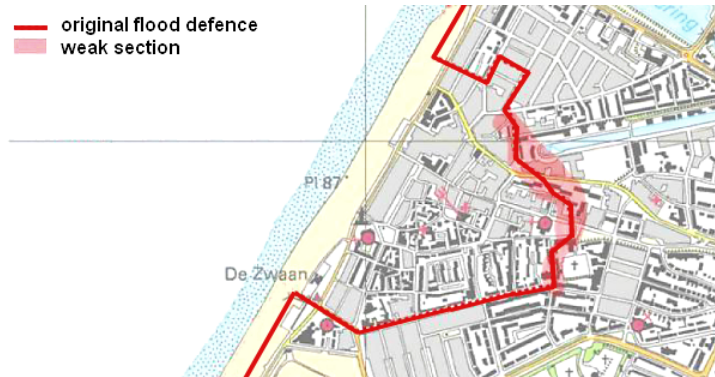
Figure 6.1: The original primary flood defence running through the town of Katwijk aan Zee (Kustwerk Katwijk, 2013)
