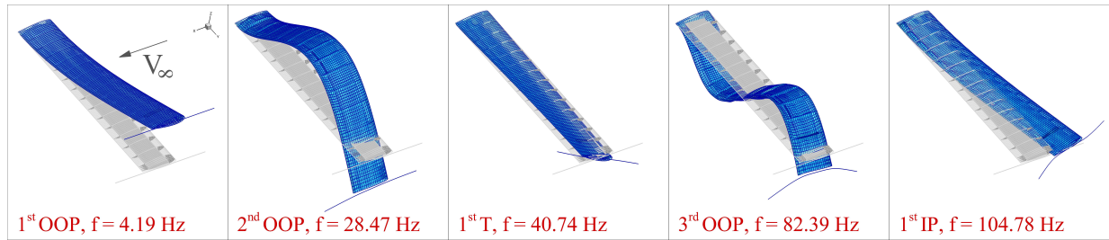
Fig. 4 Lowest five natural mode shapes as computed by MSC Nastran of the undeformed Pazy Wing full FEM with skin (OOP = Out-of-Plane bending, T = Torsion, IP = In-Plane bending).
